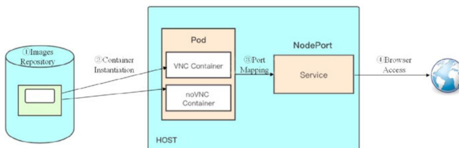
Fig. 12. Specific implement and application of the CVSimaaS.
