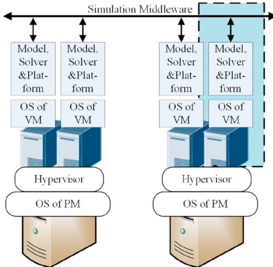
Fig. 2. Traditional VM based simulation system.
