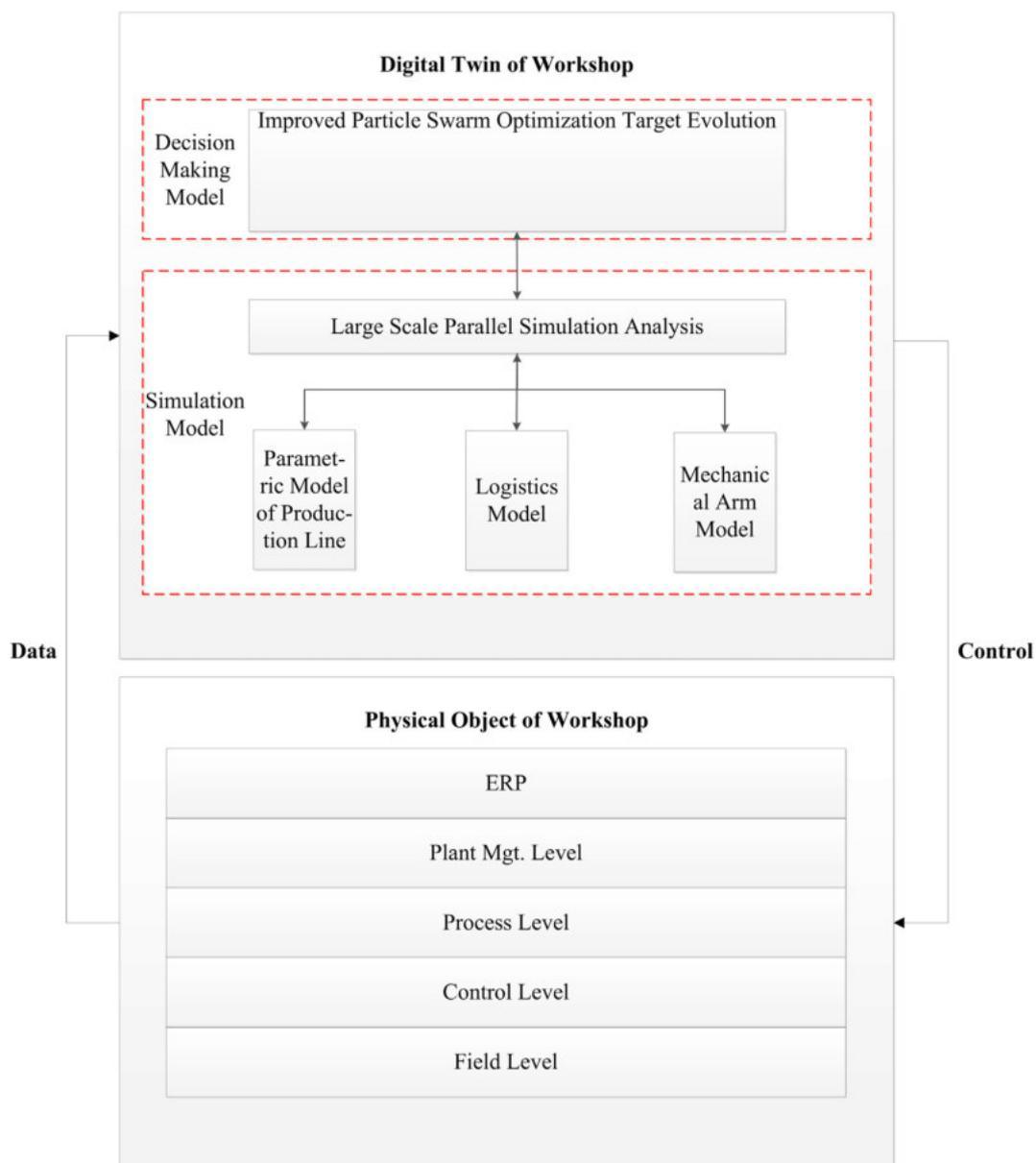
Fig. 11. A framework of intelligent manufacturing workshop scheduling application.
